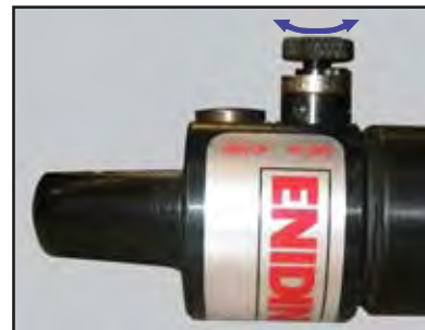
Position 0 provides minimum damping force. Position 8 provides maximum damping force. 180° adjustment with setscrew locking.
