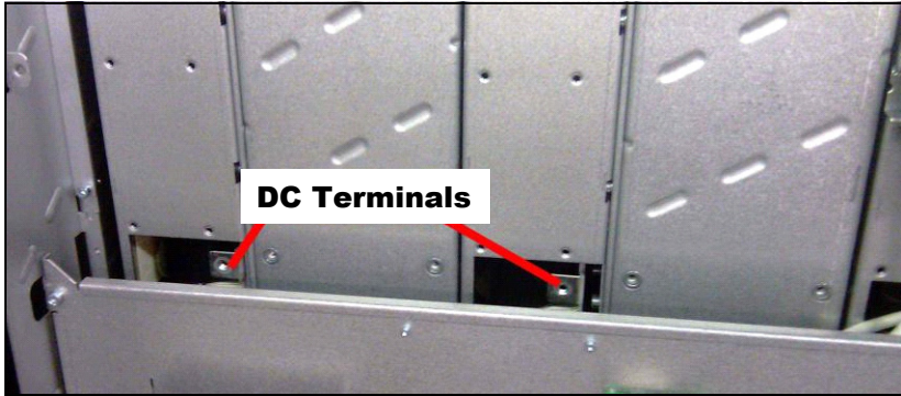
Fig. 2 Position of the DC terminals
